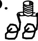
Thread the bared wires through the holes in the bulb holder, and carefully twist it around itself until firmly attached.
